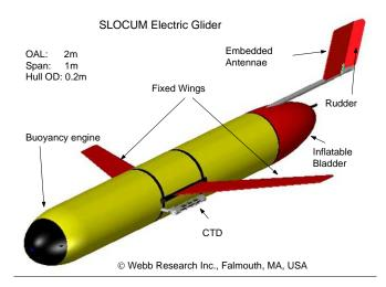
Fig. 2. Rendering of a *SLOCUM* electric glider. Built by Webb Research Inc., Falmouth, MA, USA; http://www.webbresearch.com.
